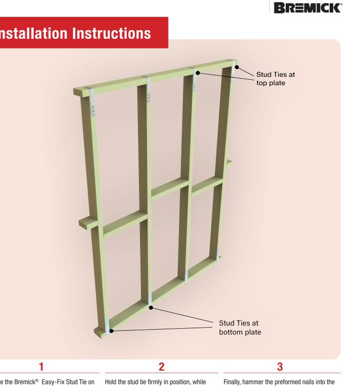
Locate the Bremick® Easy-Fix Stud Tie on the external corner of the top or bottom plate hammering the preformed nails into the of the wall frame and centrally within the stud.
