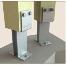
• Feed the 2 x M10 bolts through the bolt holes and timber post. Locate washer and nuts onto the bolts and tighten. A minimum of 2 x thread pitch should extend beyond the outward surface of the nut.
