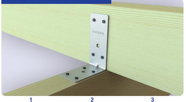
Locate the Bremick<sup>®</sup> Pergola Angle bracket, so the longest flange sits flush against the timber rafter face and the shortest flange runs along the top of the timber beam and is 35mm or 65mm timber screws through the centrally located.
